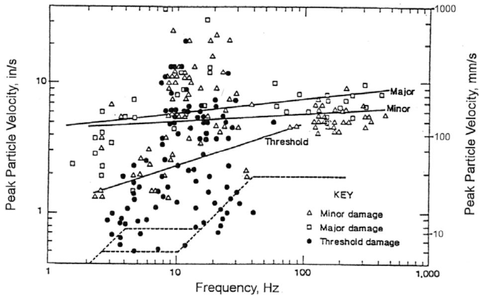
Figure 5. Ground vibration damage summary adapted from RI 8507. Dashed lines define USBM recommended safe limits. Solid lines are regressions representing data means, and symbols shown are positive damage observations. (After Siskind, 2000.)
