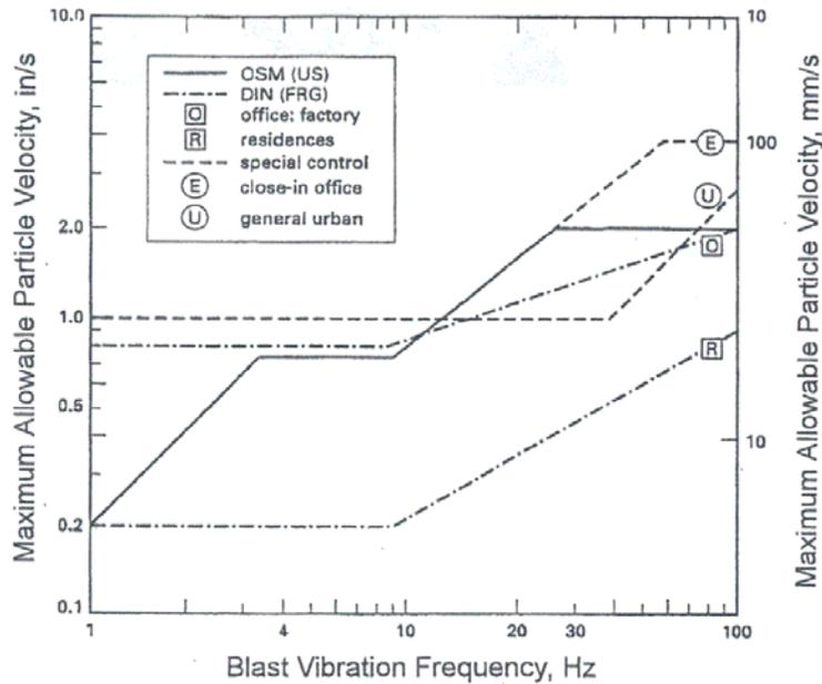
Figure 2. Comparison of different frequency-based velocity-displacement control limits. (From Dowding, 1996.)
