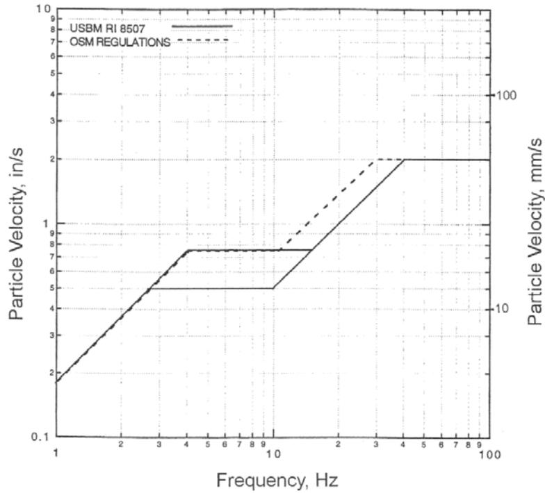
Figure 1. Safe level blasting criteria from USBM RI 8507 and OSM derivative version. (After Siskind, 2000.)
