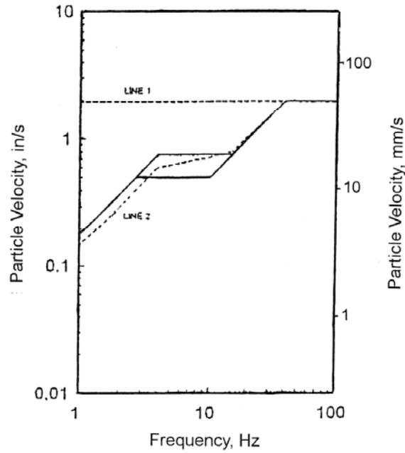
Figure 3. Vibration guidelines - USBM RI 8507 (solid line) compared to BS 7385 (dashed line). Line 1: reinforced or framed structures, industrial and heavy commercial buildings; line 2: unreinforced or light framed structures, residential or light commercial type
