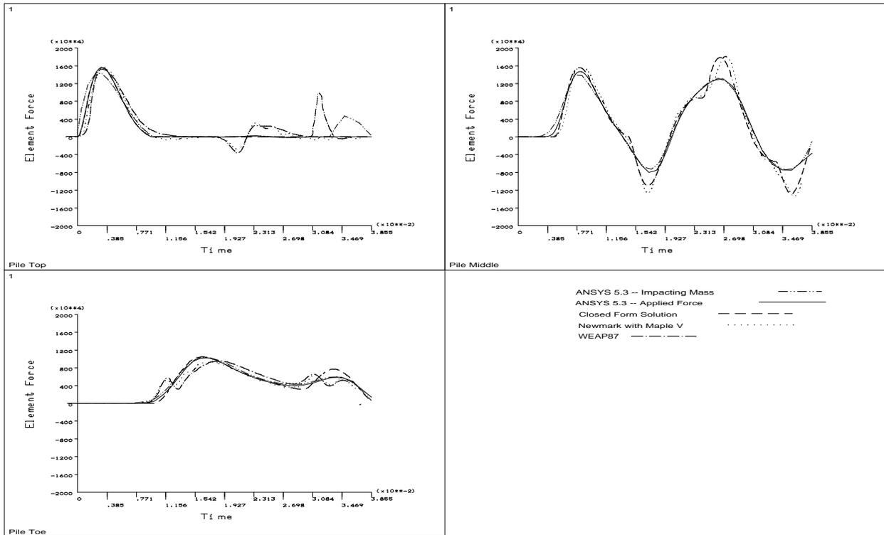
Figure 5 Comparison of Methods, Forces
