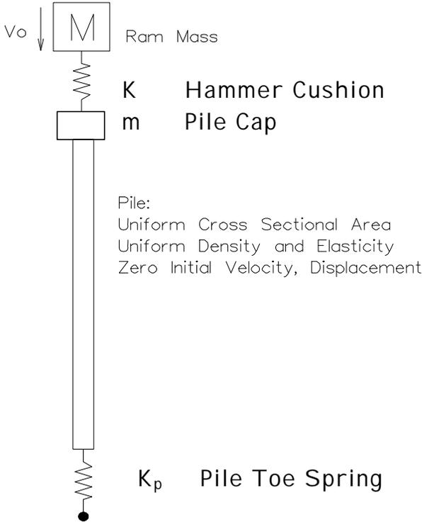
Figure 1 Hammer-Pile-Soil System
