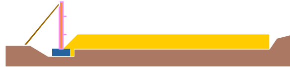
Figure 36, Fill in 6" Lifts to Reinforcement
