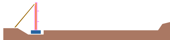
Figure 34, Install & Brace 1st Row of Panels
