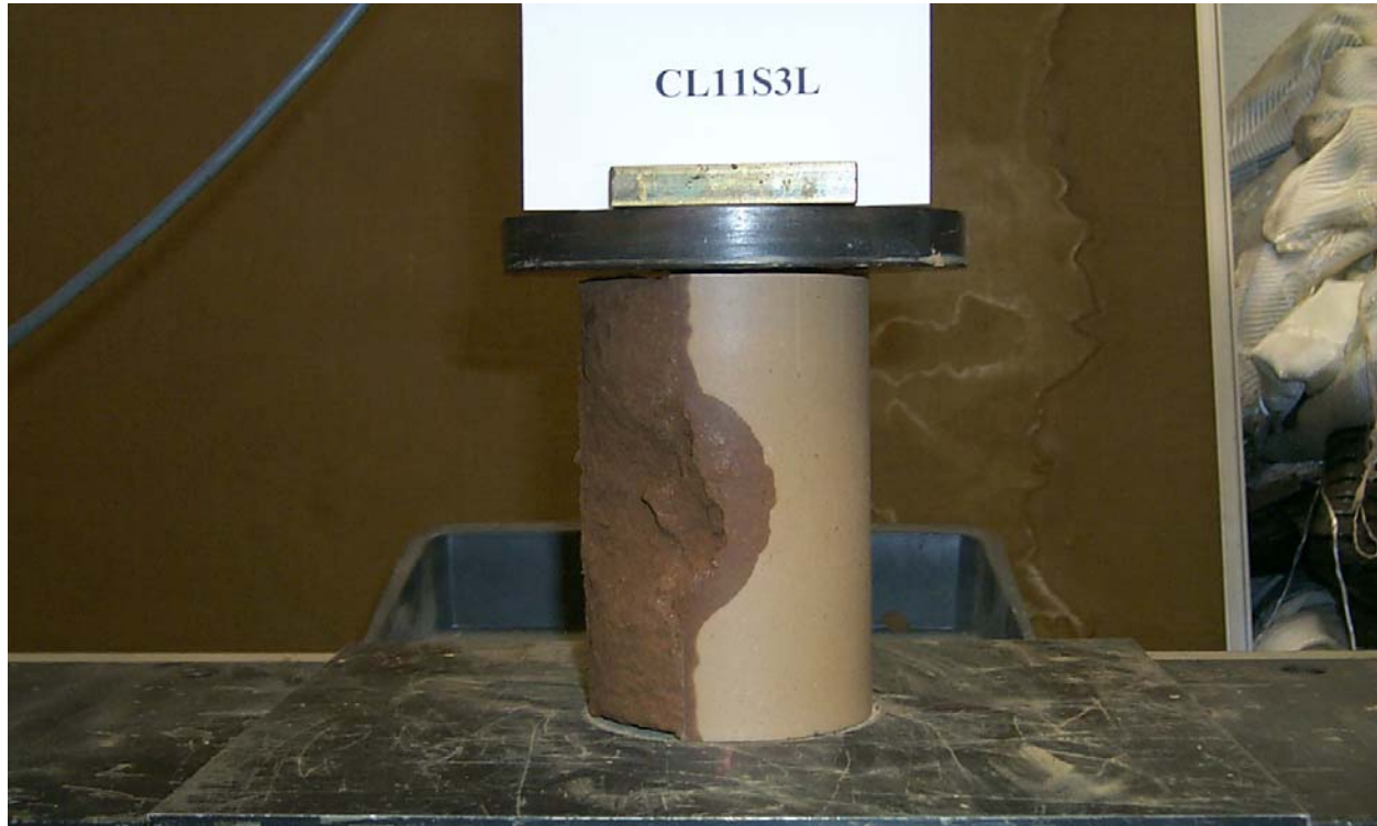
FIGURE 2 "Wet" unconfined compression test on Enzyme 2 CL specimen after soaking
