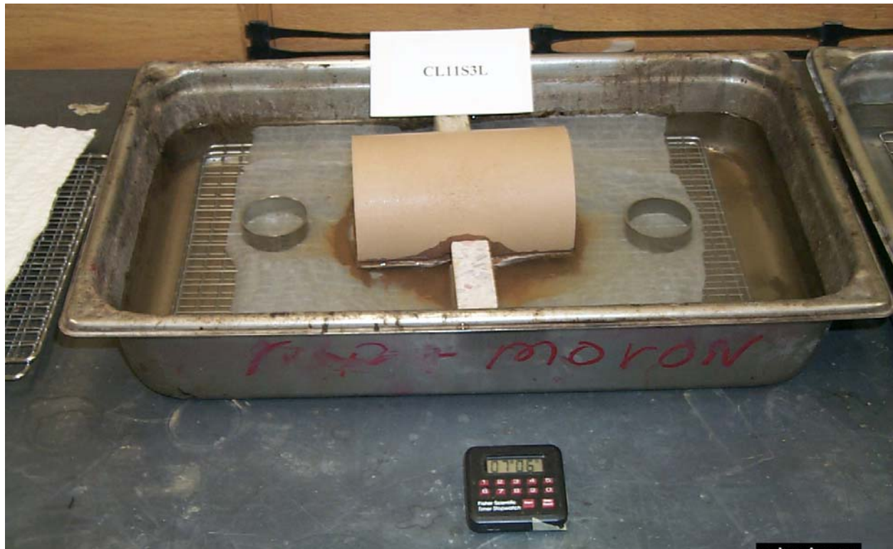
FIGURE 1 Example of Enzyme 2 CL specimen being soaked for 15 minutes
