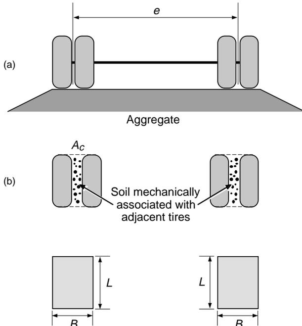
Figure 9. Definition of tire contact area for dual tires (top), and equivalent contact area used in analysis (Giroud and Noiray 1981) (bottom). (For single tires,  $L$  and  $B$  refer to length and width of single tire print, respectively.)
