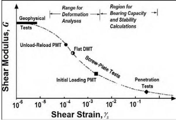
Figure 2. Typical Values of Shear Modulus Based on Field Tests (from Loehr, Lutenegeger, Rosenblad, and Boeckmann (2016))
