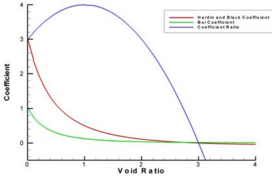
Figure 3. Comparison of Bui et al. (2010); Hardin and Black (1968) Coefficients vs. Void Ratio  $e$
