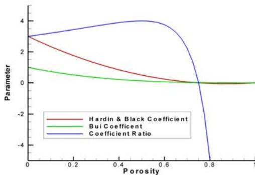
Figure 4. Comparison of Bui et al. (2010); Hardin and Black (1968) Coefficients vs. Porosity  $n$
