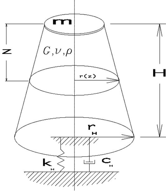
Figure 8. Pile Toe Model (from Holeyman (1988); Warrington (1997))
