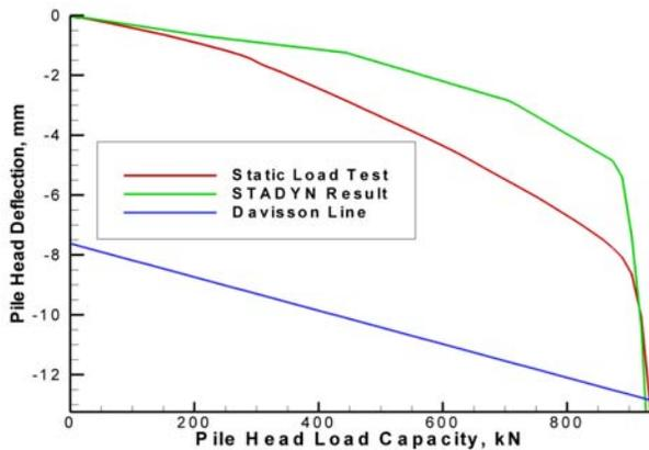
Figure 12. Comparison of STADYN Static Results with Static Load Test for Finno (1989)
