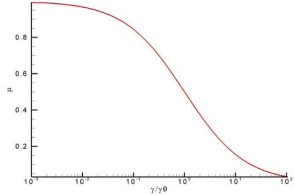
Figure 5. Softening Coefficient vs. Normalized Shear Strain (adapted from Vardanega and Bolton (2013))
