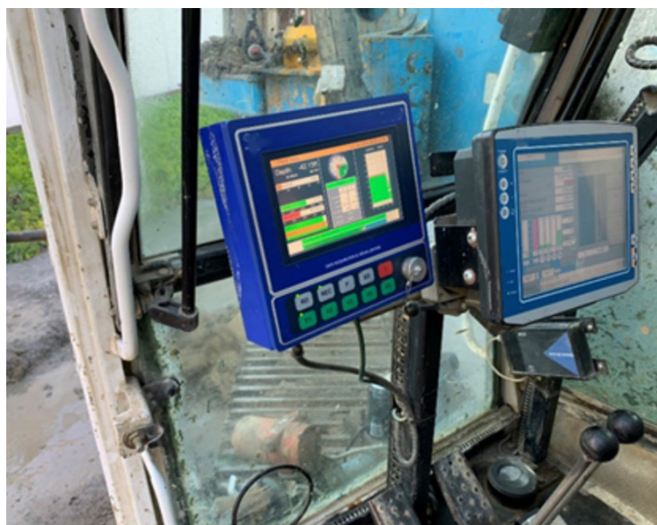
Figure 7-3 In-cab Display of Performance Monitoring System (photo by authors)
