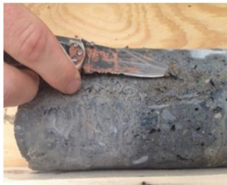
(c) Core exhibiting poor cementation
