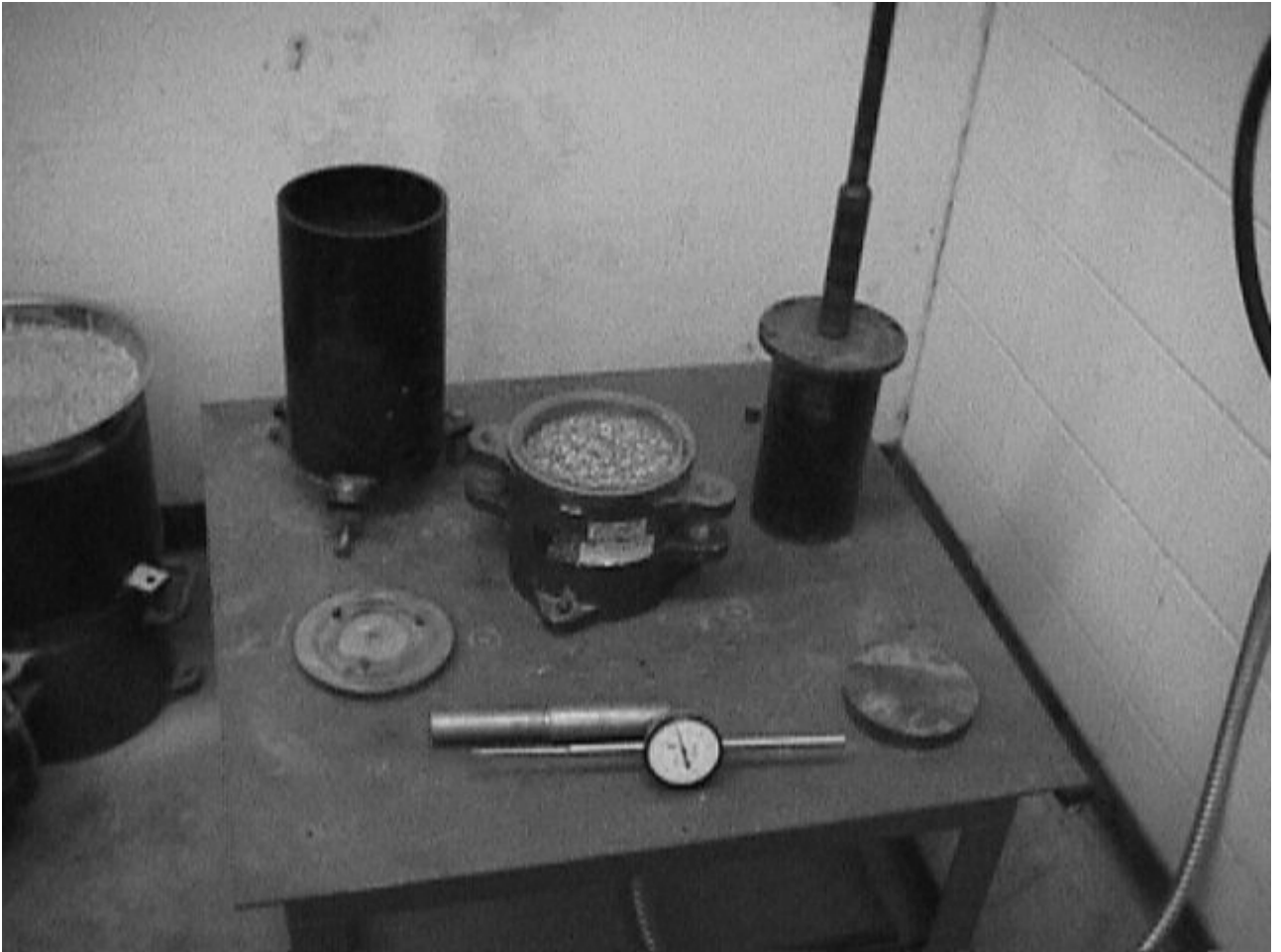
Figure 3.7: Vibratory table for Maximum Index Density (ASTM D-4253) test
